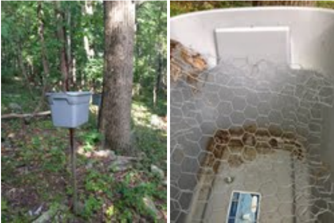
Figure 1. Seed collectors. 10 gallon plastic totes are mounted on poles and covered inside with chicken wire to prevent animal pilfering.
